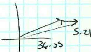
Speed =  $\sqrt{36.55^2 + 5.21^2} = \underline{37 \text{ m/s at } 8.18^\circ}$
